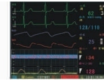
Standard interface for nine parameters: FHR, FM, TOCO, ECG, NIBP, SpO2, RESP, TEMP
